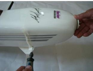
$step\ 3$  Attach the cowl using the four self-tapping screws, included in hardware pack, and a Phillips screwdriver.
