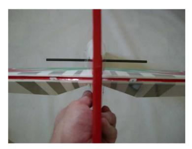
step 5Carefully place the hinges in their place, and glue the hinges with some drops of thin CA.
