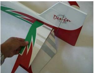
step 3With the hobby knife open the place for the carbon tube, extension and wing pin.
