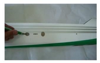
step 4Locate the carbon tube in his position and check the alignment with the stabilizer.
