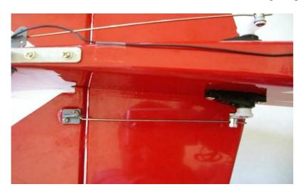
step 3Install the rudder servo and control horn into the fuselage as per picture.
