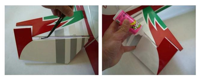
$\begin{array}{c} \textbf{step 6} \\ \textbf{Once satisfied with the alignment, glue with some drops of thin CA the stabilizer at the fuselage.} \end{array}$
