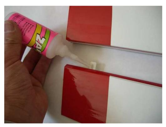
step 3Carefully glue, with some drops of thin CA, each of the four hinges into the wing panel.
