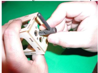
step 2Locate the engine mount on the fuselage and glue it with medium CA.
